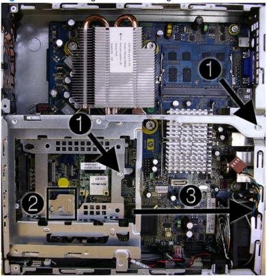
Figure 7-26 Removing the hard drive cage
